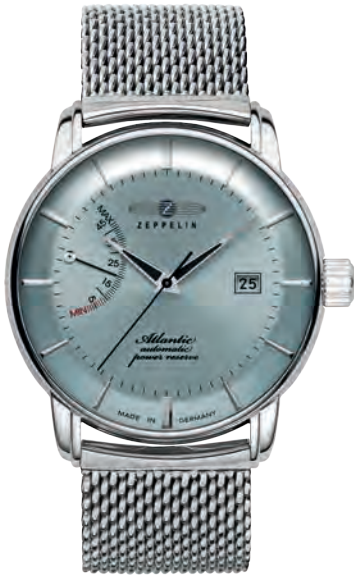
8462M-6 | Automatik mit Gangreserveanzeige Automatic with Power Reserve Indicator Citizen-Miyota 9133 | 26 Jewels | Date | Mineral Crystal K1 | Crystal Exhibition Back | wr 5 atm | Ø 42 mm
